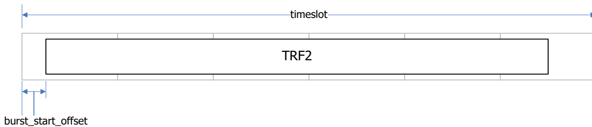
Figure 7-30: Example of a Burst in a Timeslot Built from 6 BTUs
