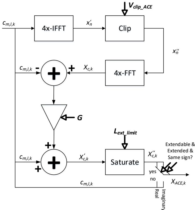
The diagram in the specification (figure 50) shows processes of IFFT, four-times oversampling and low-pass filtering, but the text explains that these three processes are done using a “four-times oversized IFFT operator”. The figure above is a modified version of figure 50 with this operator replacing the separate notional processes (and with the corresponding 4x-FFT – see below). The definition of this operator is as follows:
